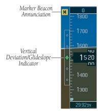
Figure 2-8 Marker Beacon and Vertical Deviation
