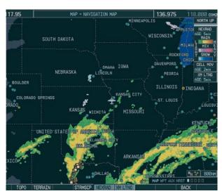
Figure 10-7 Navigation Map Page Displaying NEXRAD Weather
