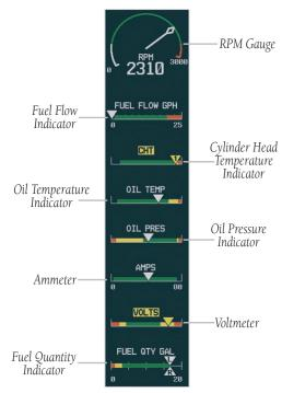
Figure 3-2 DA 40 F (Fixed Pitch Propeller)
