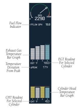
Figure 3-4 DA 40 F (Fixed Pitch Propeller) LEAN Engine Page
