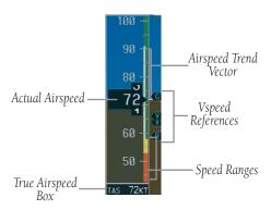
Figure 2-4 Airspeed Indicator
