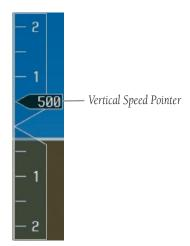
Figure 2-9 Vertical Speed Indicator
