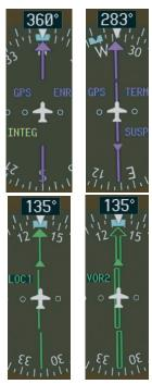
Figure 2-18 GPS INTEG, GPS SUSP, LOC1 and VOR2
