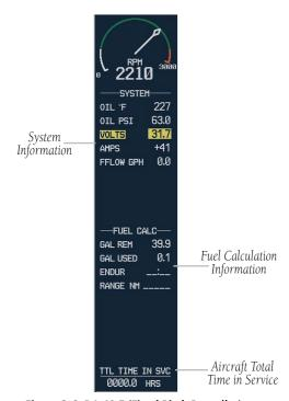
Figure 3-6 DA 40 F (Fixed Pitch Propeller) SYSTEM Engine Page
