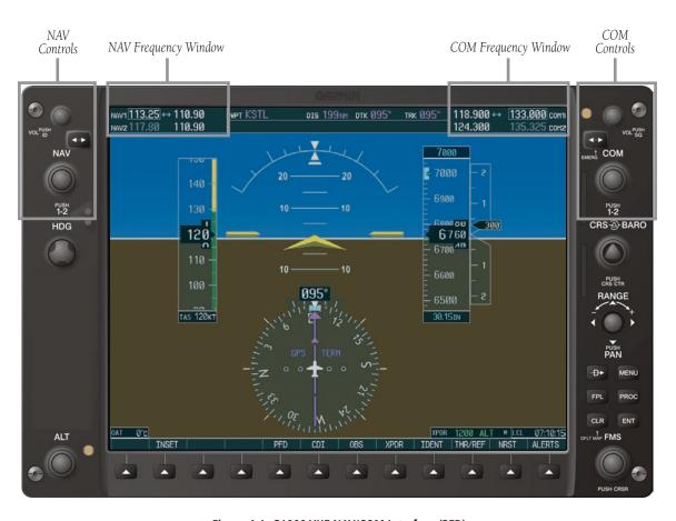
Figure 4-1 G1000 VHF NAV/COM Interface (PFD)
