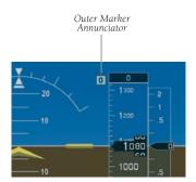
Figure 5-3 Marker Beacon Signal Indicator Lights on the PFD
